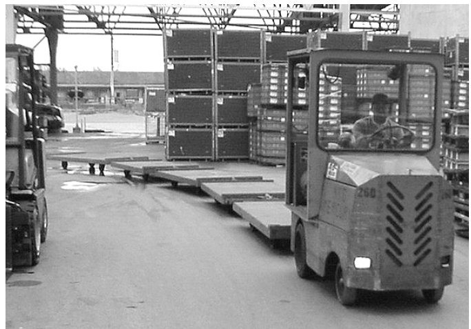
Assembly line delivery trailers with 80 Series casters built to automotive specifications.
